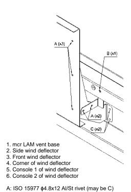
B. ISO 15977 φ6.4x12 Al/St rivet C. ISO 15973 φ4.8x12 Al/St rivet (sealed)
