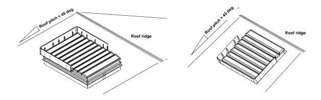
mcr LAM louvered vents can be mounted on steel, concrete or timber roofs. The additional lower base, the roof curb, features a ledge at its bottom to support and secure the vent to the supporting structure. The fasteners should be appropriate to the supporting structure material (steel, concrete, timber) and not smaller than 6 mm in diameter. The intervals between fasteners should not be greater than  $50 \div 60$  cm.
