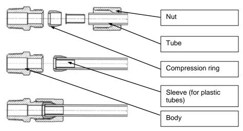
Figure 15. Connection of union with a copper/steel air tube.
